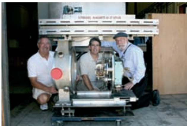
SLAC equipment being sent to SESAME. In the rear is the PEP 2 m long permanent magnet undulator. In front is the water-cooled double-crystal Brown-Hower X-ray monochromator (left to right are Richard Boyce, Charles Troxel Jr., and Herman Winick from SLAC) (Photo by courtesy of Stanford Linear Accelerator Center (SLAC) in the USA)
