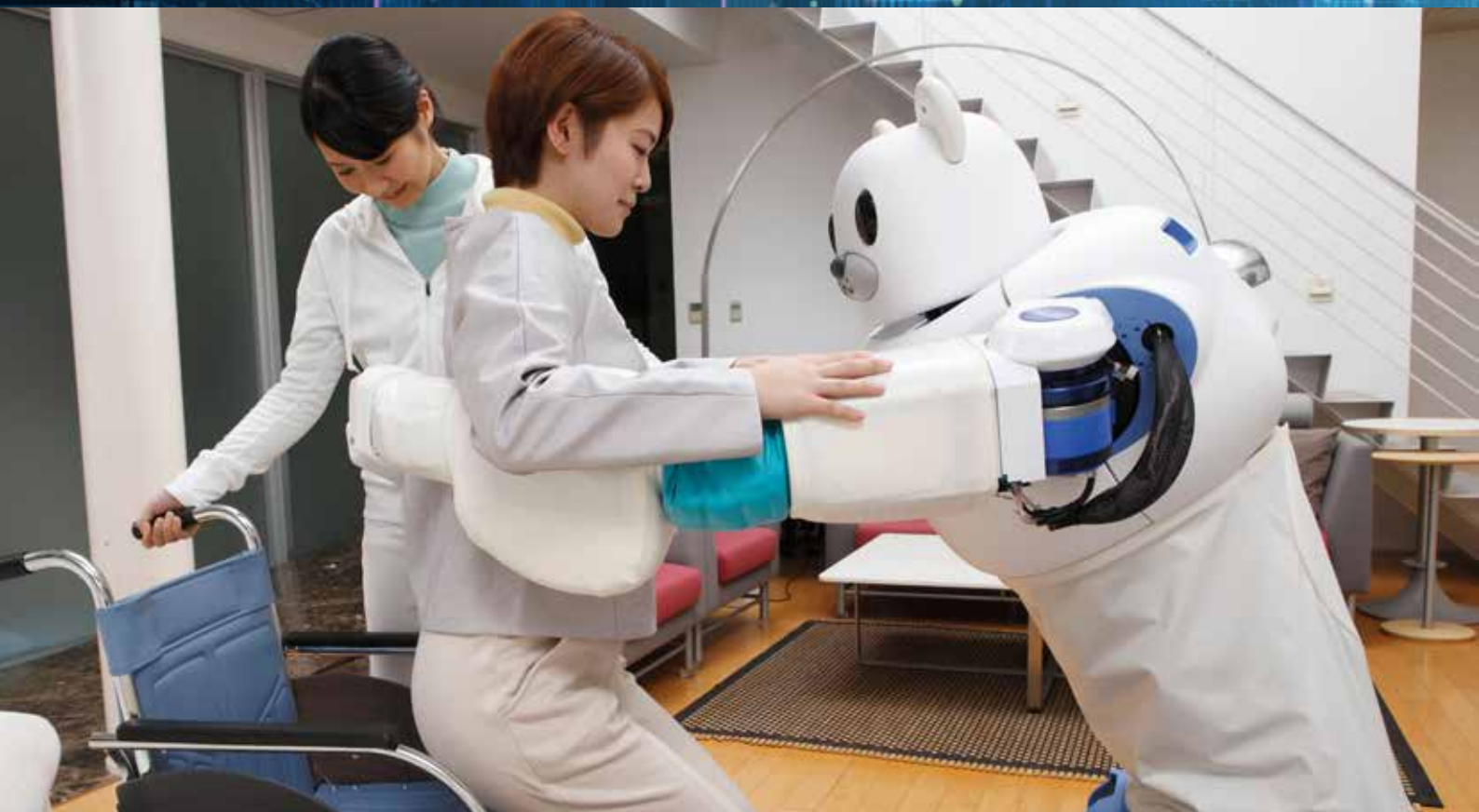
ROBEAR has been developed by RIKEN as an experimental project to see if robots can be used to help people with restricted mobility move between their wheelchair and other furniture. It is capable of carrying a reclining adult in its arms and can travel in different directions. © RIKEN
