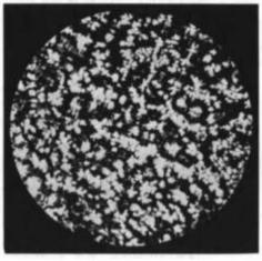
PLATE 9.2 Microphoto of a section in a copper staple from the Cheops Boat at Giza showing the fragmented dendritic character due to hammering
