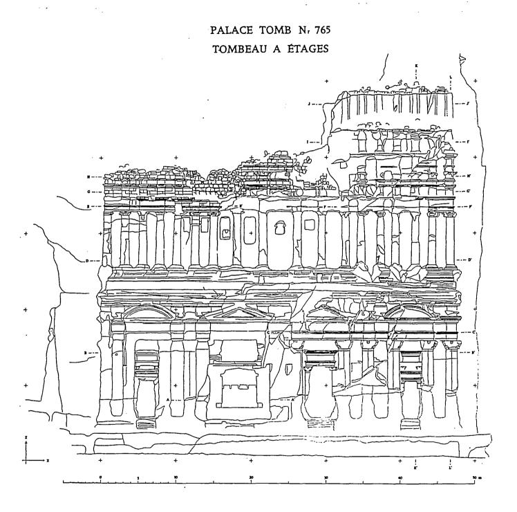
Fig. 15. Photogrammetric survey by IGN of the Palace Tomb Facade
