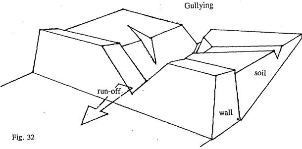
Gullying of the terraces following the destruction of a retaining wall. Rewerski
